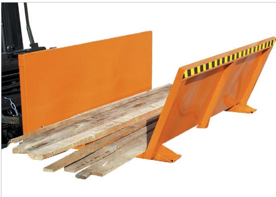
**Container used to collect and tip out materials such as strips of wood, planks, plastic profiles, metal rods**
