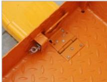
Safety mechanism for a straddle stacker
