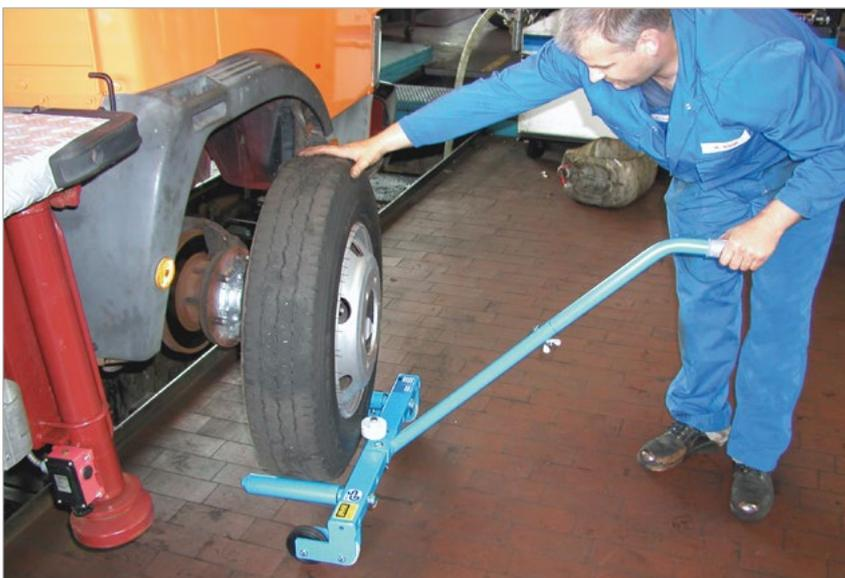
Easy tyre fitting for trucks, buses and forklift trucks
