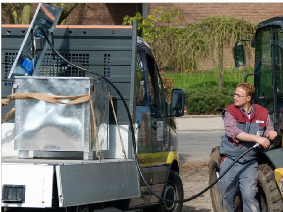
Mobile, single-walled tank for diesel and fuel oil supply for building site vehicles and machinery. ADR 1.1.3.1. c) compliant (exemptions related to the nature of the transport operation).
