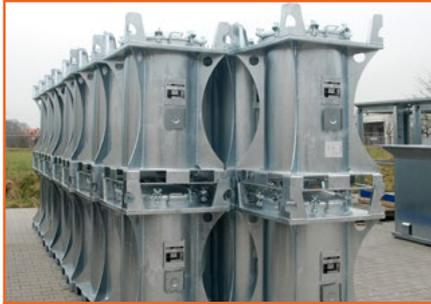
**Special Waste Containers for solids, paste-like substances and hazardous liquids** 146
