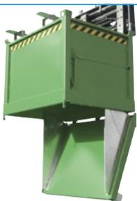
Containers emptied via a trap door are compact in design but also high capacity. An optimised load centre means maximum utilisation of the forklift load capacity. A pull cable operates the base which opens wide; thanks to the large aperture the load is fully discharged every time - even bulky materials.
