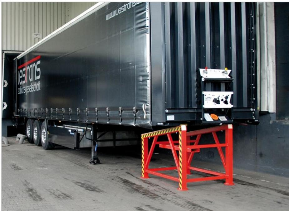
**Loading support to facilitate loading and unloading articulated trucks up to 25 tonnes**
