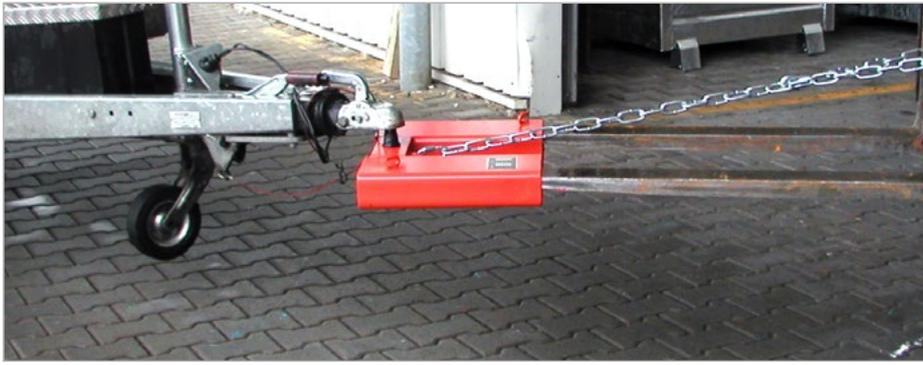
**A shunting aid makes light work of manoeuvring trailers on company premises, for example on the shop floor**
