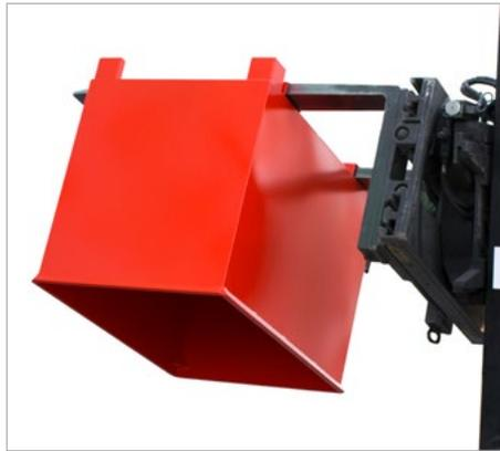
Emptying using a forklift rotator
