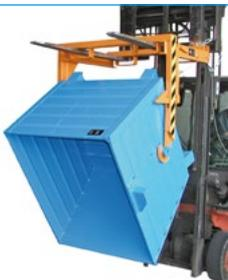
These containers are an economical alternative as they do not have a built-in emptying mechanism. Any number of containers - providing they are the same width - can be picked up by one and the same traverse. Containers without pins must be discharged using a forklift rotator.
