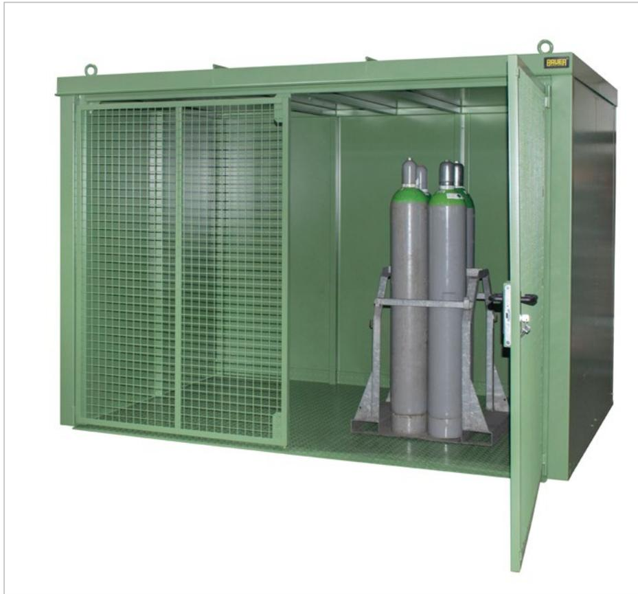
**Outdoor storage of gas cylinders, fully assembled, F90 fire-resistant walls and roof; DIN 4102 compliant**
